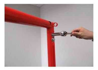
5. Slip (1) 3/8" x 1" CARRIAGE BOLT thru the open hole of the HEADER BAR NET LACING STRAP at both ends. Loosely connect CARRIAGE BOLT to STRAP using (1) 3/8" LOCK WASHER and (1) 3/8" WING NUT. Slip head of CARRIAGE BOLT through the "T" slots on the HEADER BAR as shown below. When head of CARRIAGE BOLT is proper seated into the bottom of all four "T" slots, hand tighten WING NUTS.
