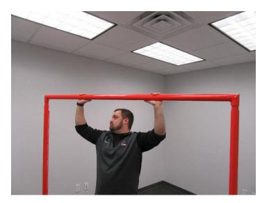
4. Connect the HEADER BAR to the UPRIGHTS by screwing (2) 3/8" x 3/4" HEX BOLT, (2) 3/8" LOCK WASHER, and (2) 3/8" FLAT WASHER into the threaded holes on the HEADER BAR as shown. Repeat this step to complete the other side.
