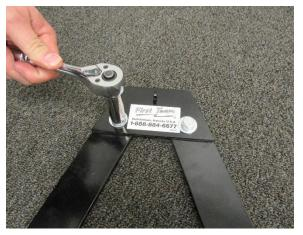
2. Loosely Screw (1) 3/8" x 3/4" HEX BOLT, (1) 3/8" LOCK WASHER, and (1) 3/8" FLAT WASHER into the threaded hole on the GROUND BAR sleeve. Then slide the UPPICHT over the GROUND BAR sleeve and tighten. Repeat steps for opposite side.
